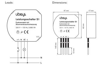
For installation of the power switch S1, the included clamps can be used. The power switch S1 retains its switch position when disconnected from power. The switch position is undefined by delivery; i. e. the switching output can be conductively connected to the phase L!
