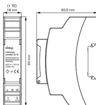
The power switch S1-R retains its switch position when disconnected from power. The switch position is undefined by delivery; i. e. the switching output can be conductively connected to the phase L! During installation, the general risks of household voltage networks have to be noted!
