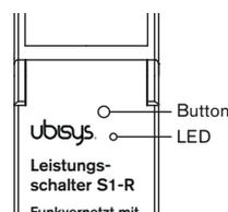
\*) If the device has legacy firmware this feature might not be available. In this case, keep the button pressed for one second, until the LED flashes three times and then blinks once every second. Then press the button four times for less than a second, until the LED flashes five times, followed by a pause, then flashes five times again, followed by a pause, etc. In this state, keep the button pressed for more than a second until the LED starts flashing rapidly.
