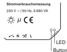
\*) If the device has legacy firmware this feature might not be available. In this case, keep the button pressed for one second, until the LED flashes three times and then blinks once every second. Then press the button four times for less than a second, until the LED flashes five times, followed by a pause, then flashes five times again, followed by a pause, etc. In this state, keep the button pressed for more than a second until the LED starts flashing rapidly.
