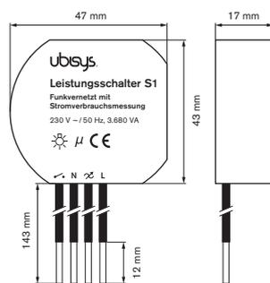
For installation of the power switch S1, the included clamps can be used. The power switch S1 retains its switch position when disconnected from power. The switch position is undefined by delivery; i. e. the switching output can be conductively connected to the phase L! During installation, the general risks of household voltage networks have to be noted!
