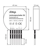
For installation of the power switch S2, the included clamps can be used. During installation, the general risks of household voltage networks have to be noted!
