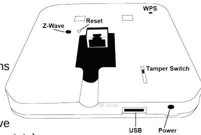
The HUB provides 4 buttons on the backside of the enclosure:
